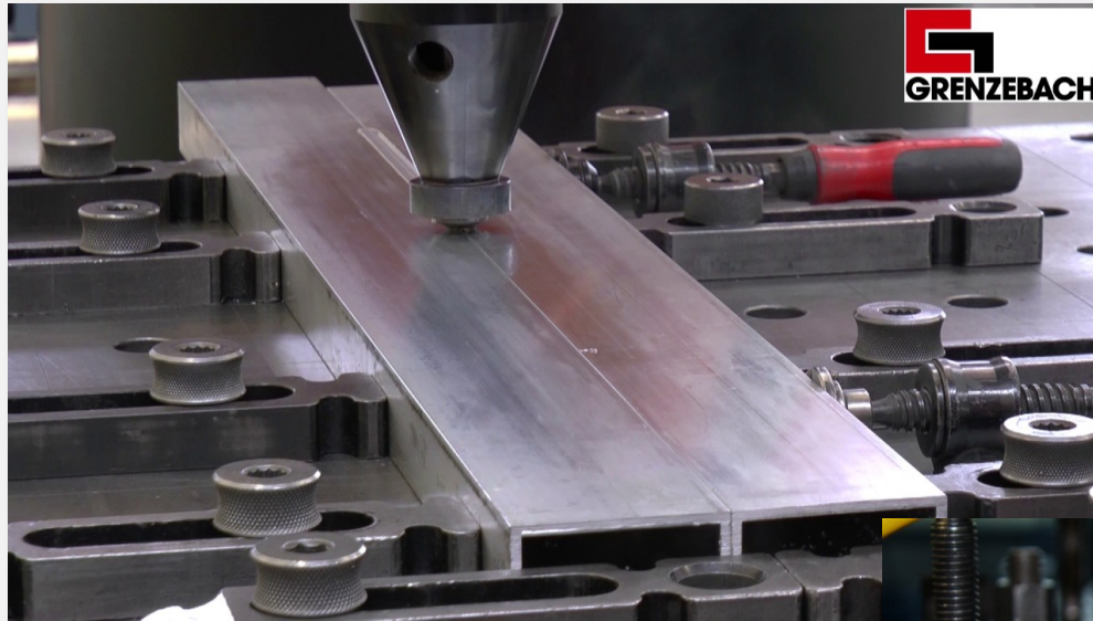
FSW weld – Without edge preparation
