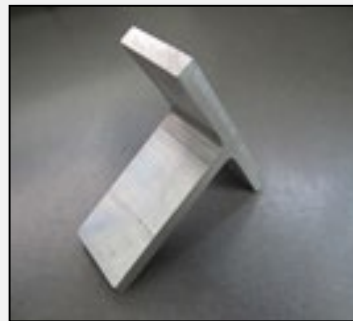
8 mm thickness Al-alloy Corner Seam Sample welded by stationary shoulder FSW
