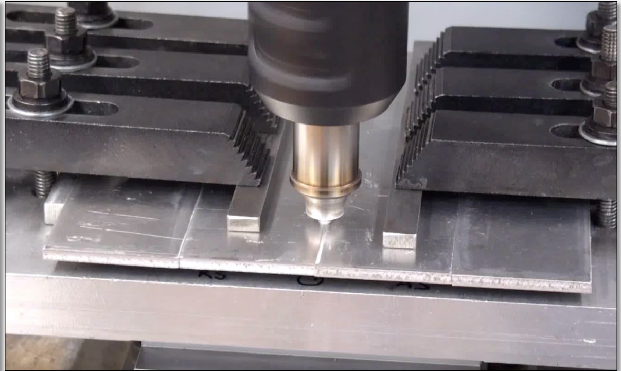
FSW weld – Without edge preparation
