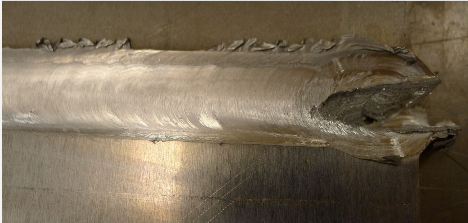
Run-out of welding tool without a splice plate
