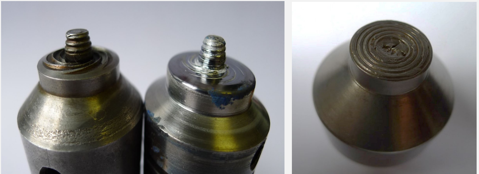
The worn-out welding tools made of steel type 19554 (H13)
