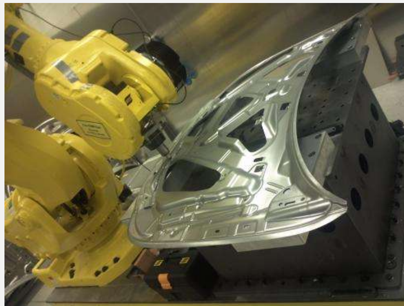
Robotic FSW of car body panel
