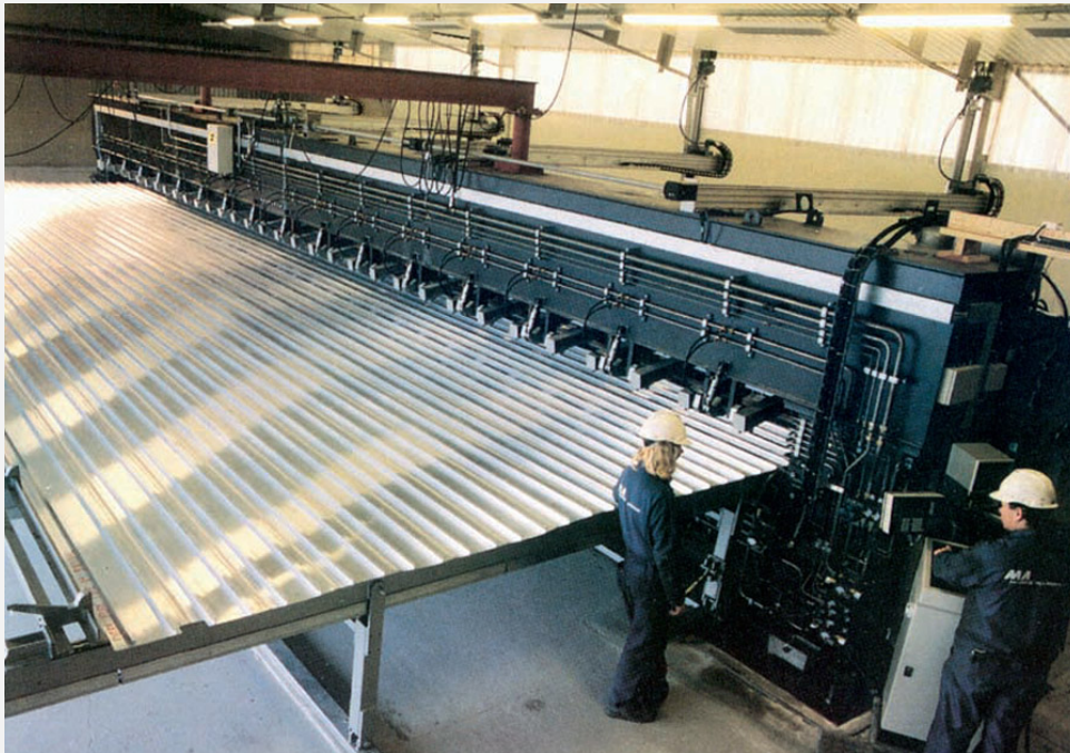
Shipbuilding – large panel FSW
