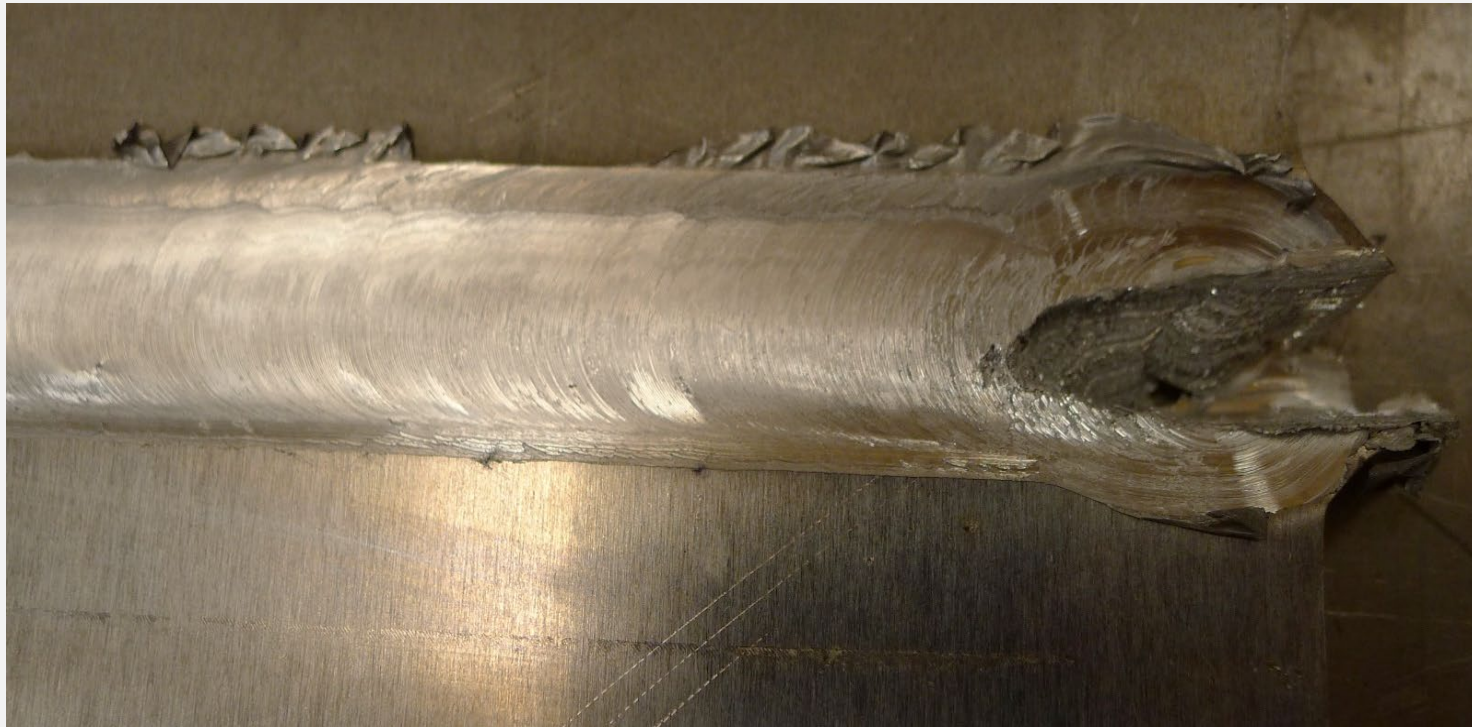
An imprint from welding tool
