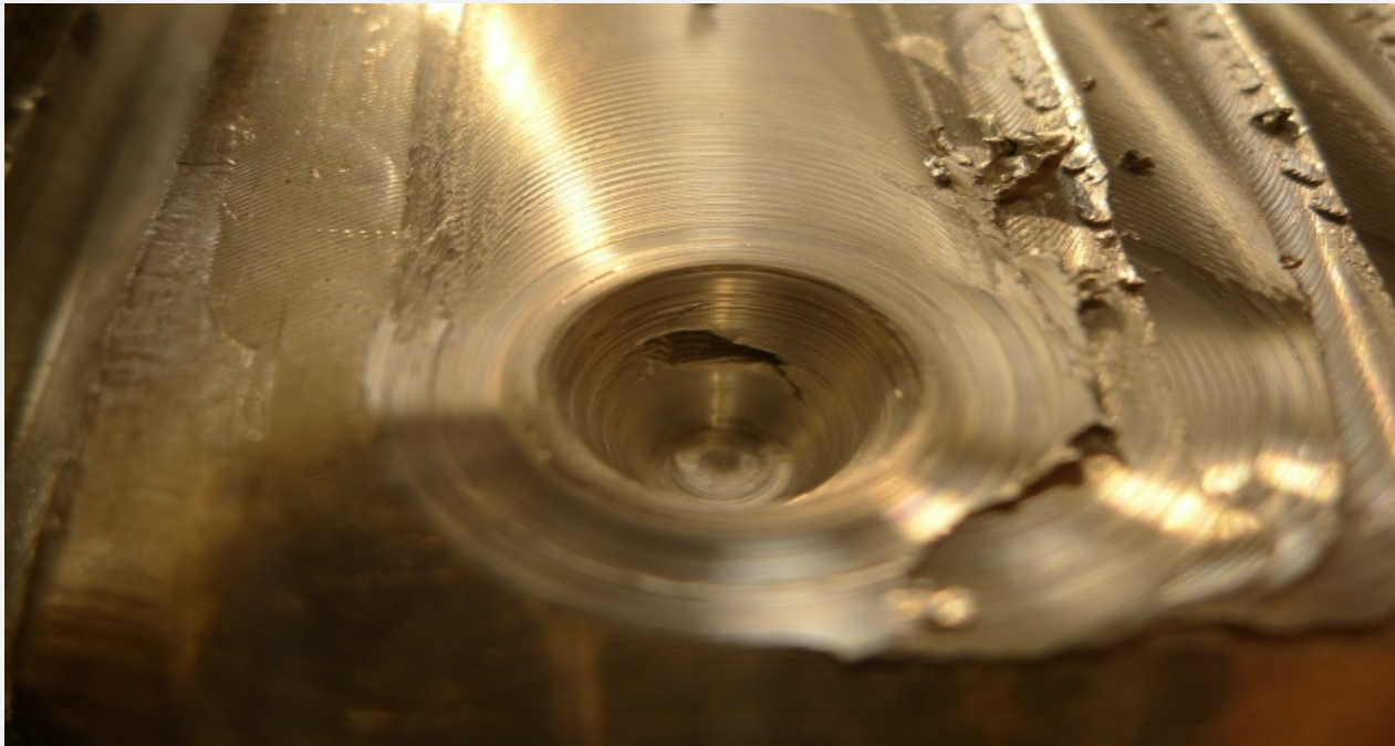
Sub surface voids Al alloys
