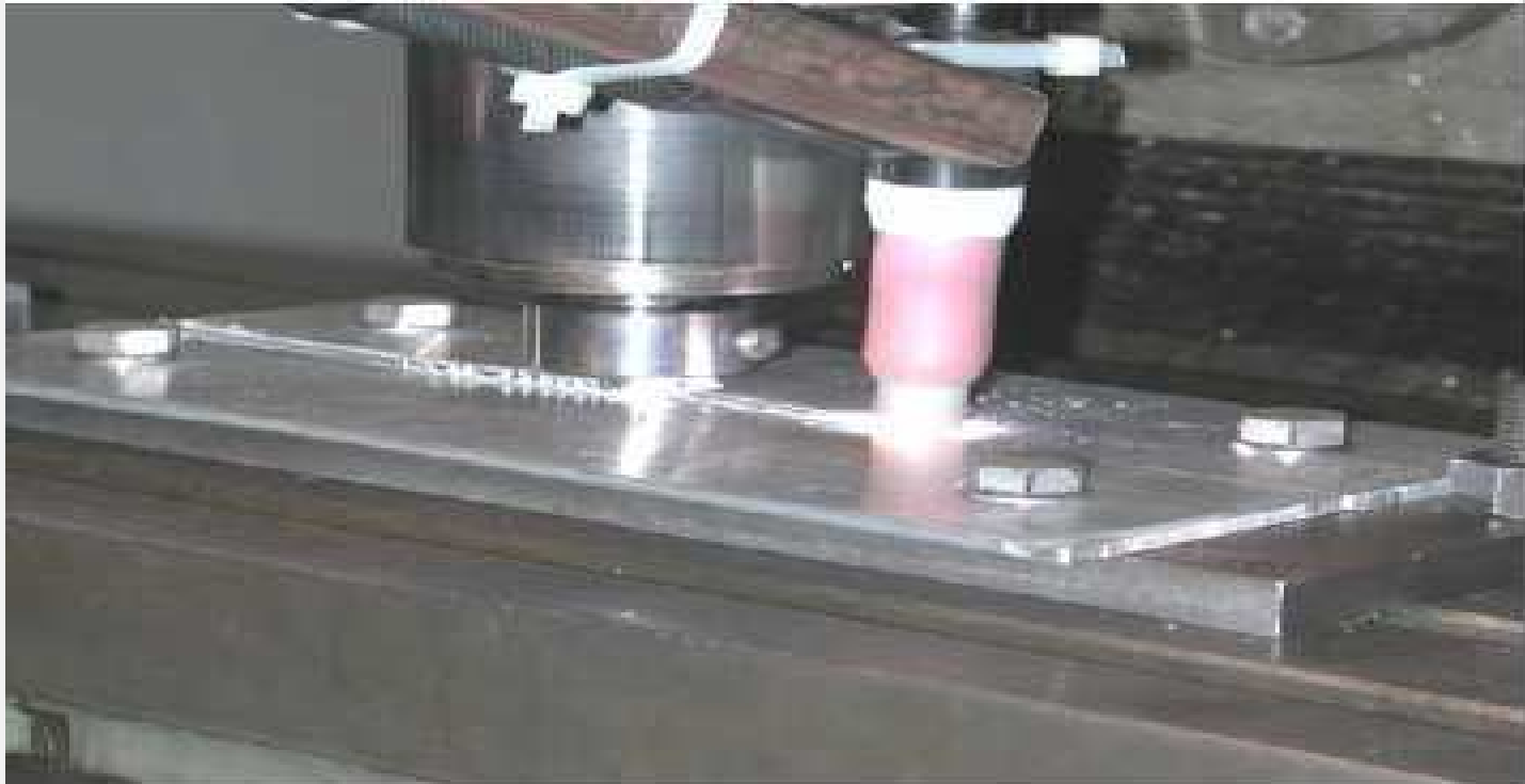
HFSW equipment with participation of a GTAW heat source
