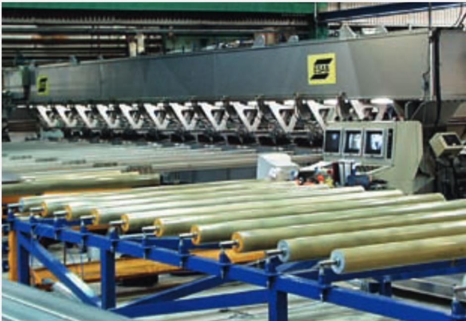
Railway – fully automatic extruded profile panels welding
