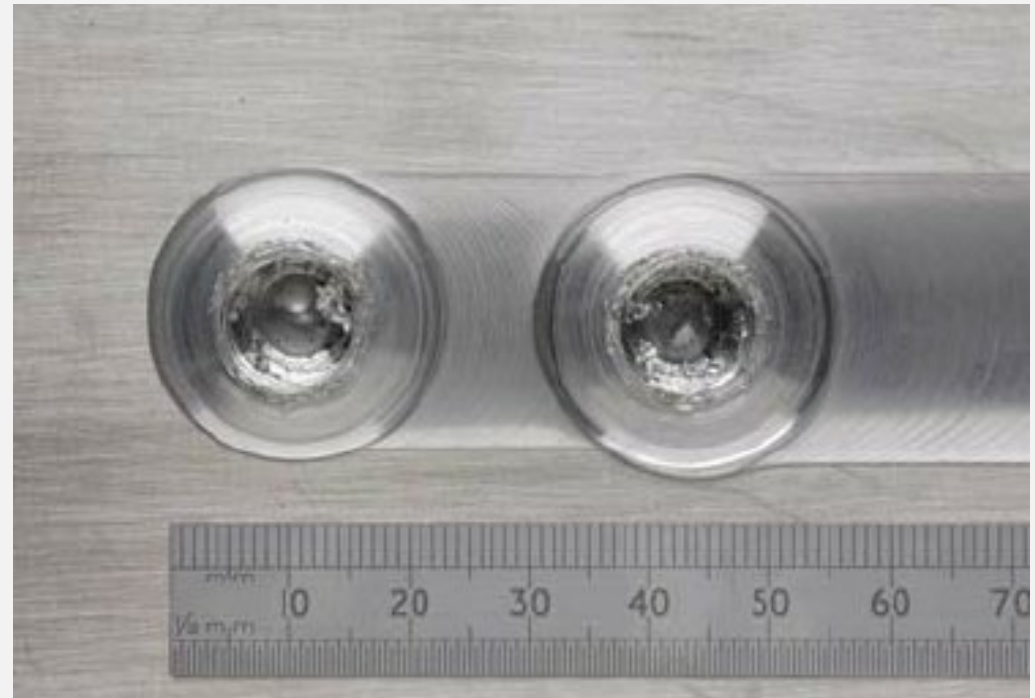
Tandem FSW exit holes
