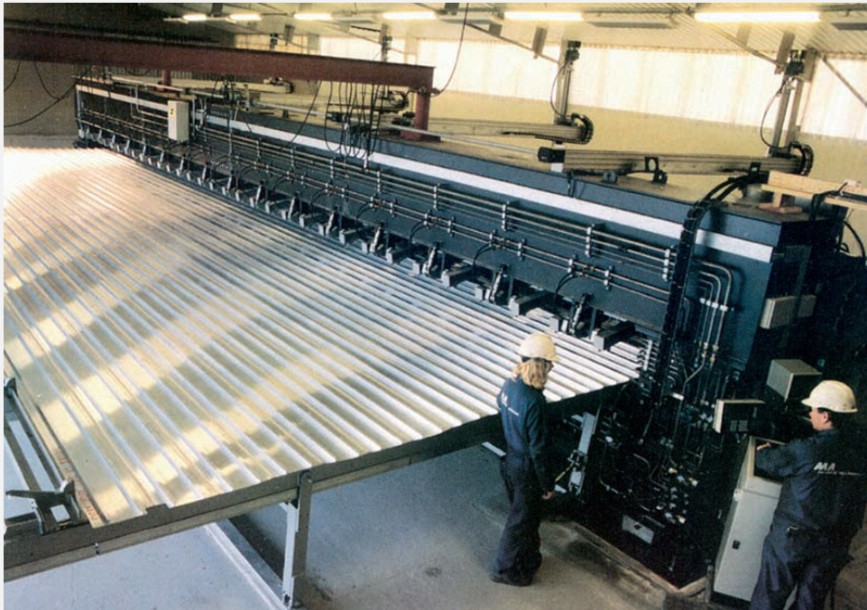
Shipbuilding – large panel FSW
